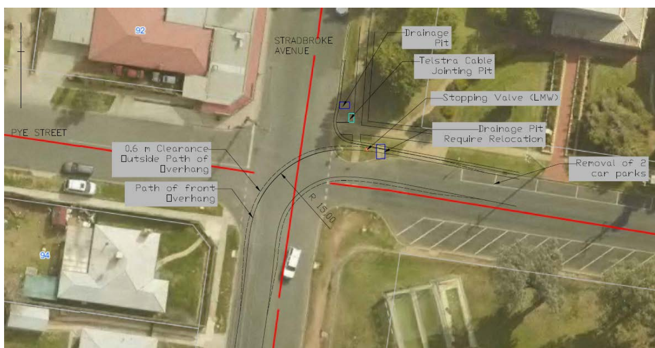
Figure 2. Concept design of lane widening at Pye Street.
