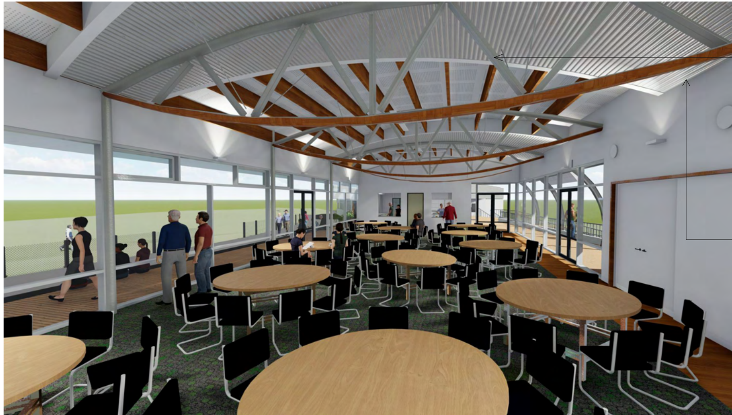
Galvanised Steel Trusses: Equal Angles – cleats connections
