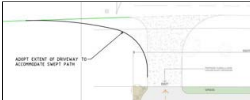
Figure 7: Proposed driveway modifications for left turn exit movements by trucks
