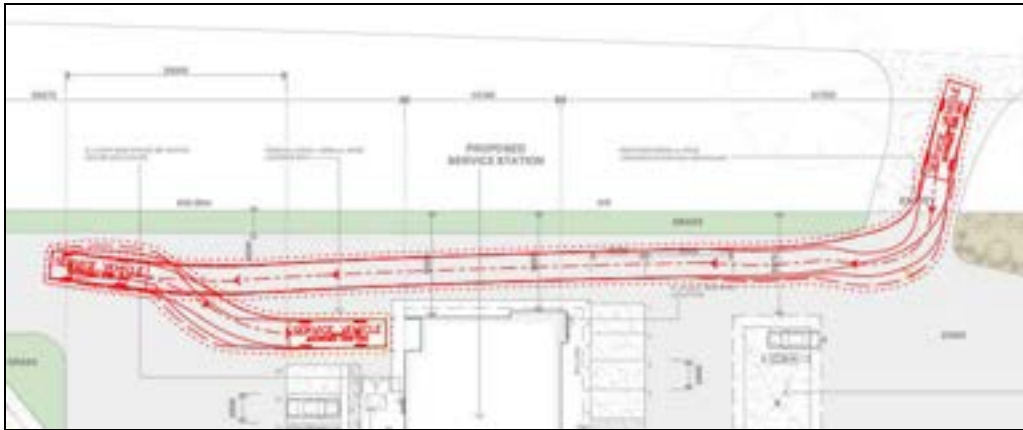
Figures B3 & B4: Swept path plots for 8.8 m service vehicle accessing the delivery dock.
