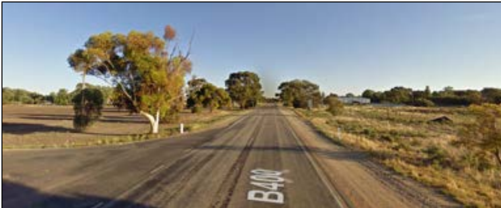
Photo 4: View to the north from the proposed exit driveway for the subject site showing compliance with Austroads SISD criteria
